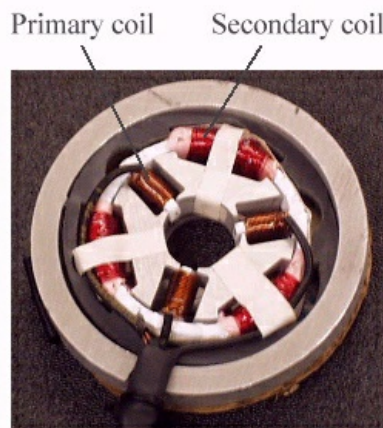
A Three-Phase Sensor, opened to show three primary coils on the poles, and three secondary coils on the ring
