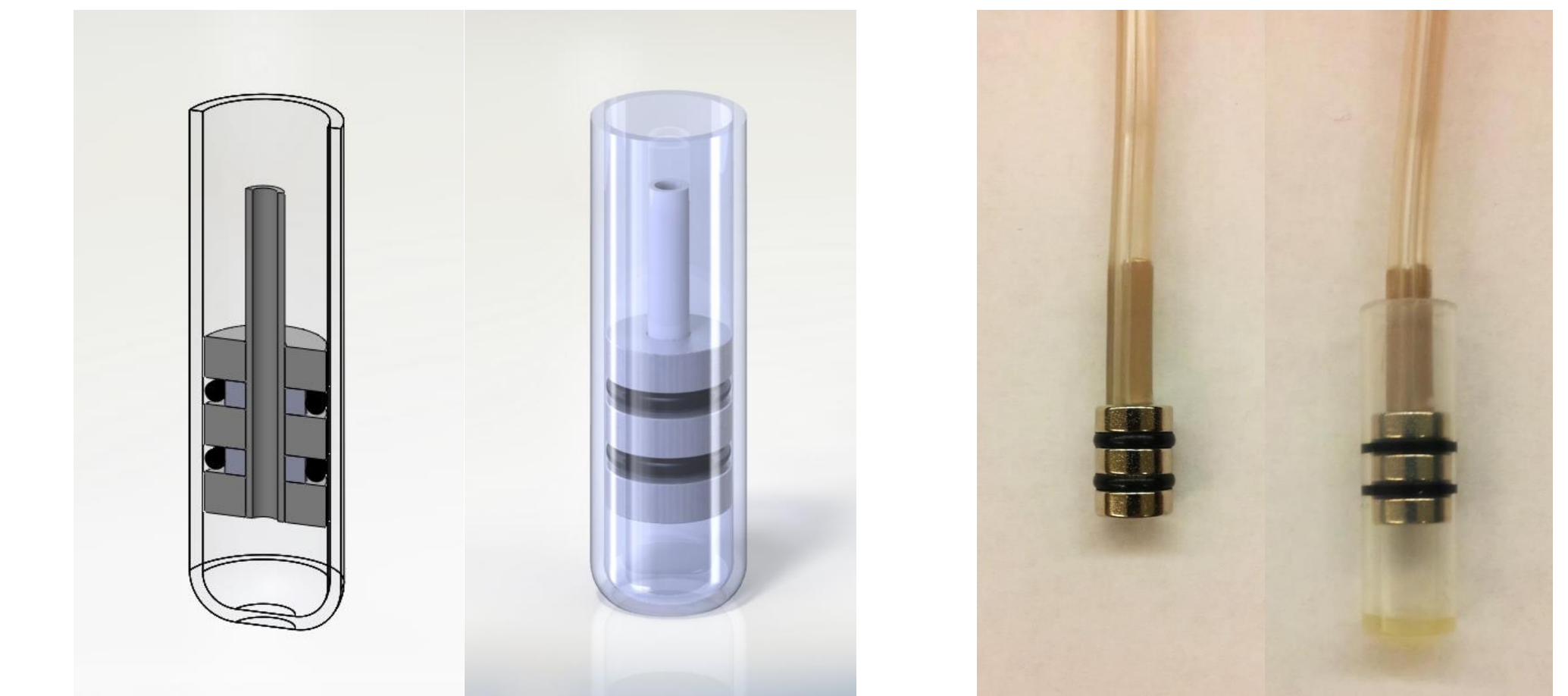
End-effector Assembly consisting of barrel and magnet plunger. Magnet plunger is comprised of ring type NdFeB magnets, O-rings, spacers, and tube for injecting fluid.
